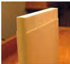
Giant tenon. The key is to start with a giant tenon with a narrow shoulder.
